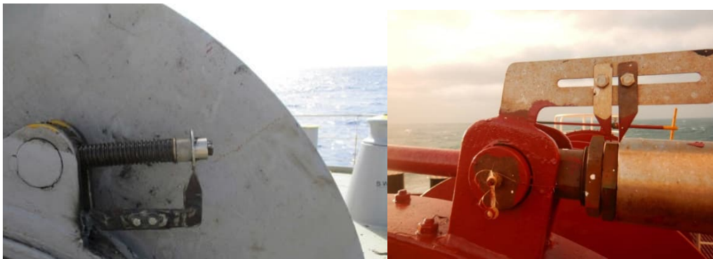
Fig 11: Mooring Winch Brake Correct Setting/Alignment.
