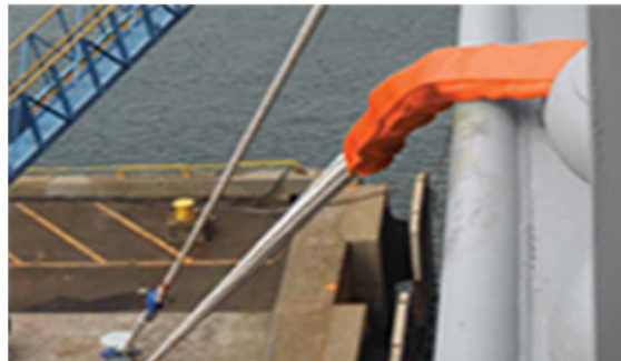
Fig 16: Mooring Line chafe protection.
